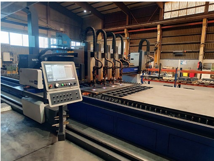
Caption 2: The easy-to-use machine control Global Connect on the ELEMENT with oxyfuel machine torch ALFA and extraction table, © Wagner Stahl
