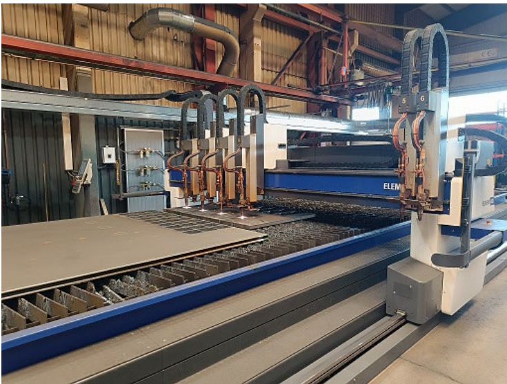
Caption 3: Four of the six oxyfuel machine torches ALFA in action on the ELEMENT, © Wagner Stahl
