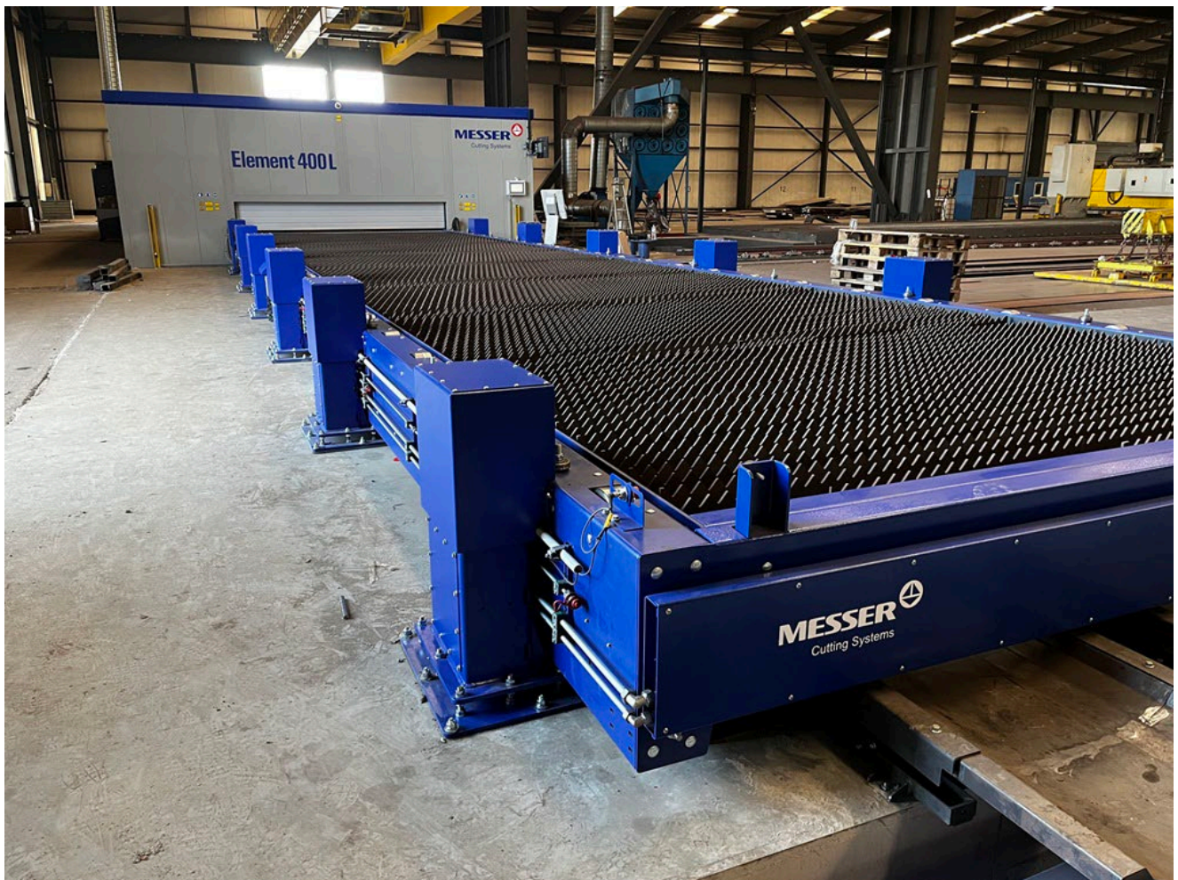
Image 1: With cutting, changing and loading table, the ELEMENT L reaches a length of 60 meters.
