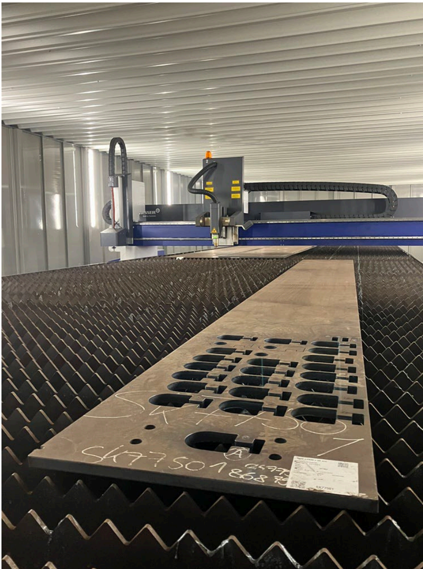
Image 2: The ELEMENT L is equipped with a needle marker and bevel cutting head Bevel-U.
