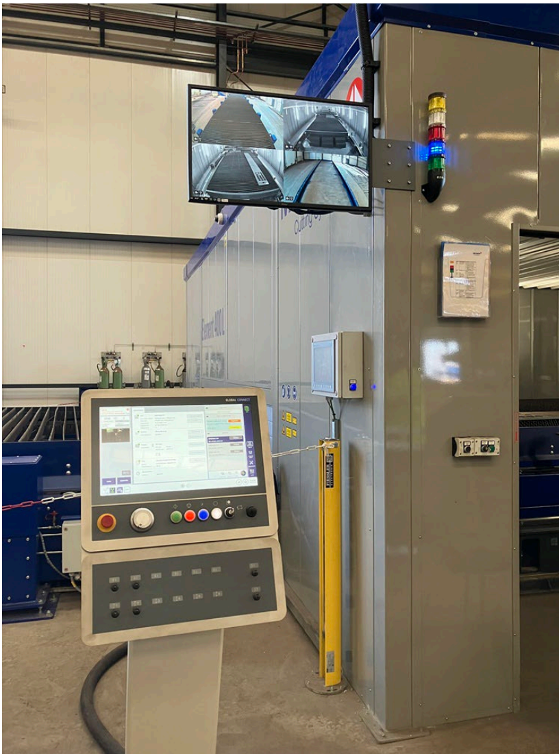
Image 3: State-of-the-art CNC control with Global Connect and video surveillance.
