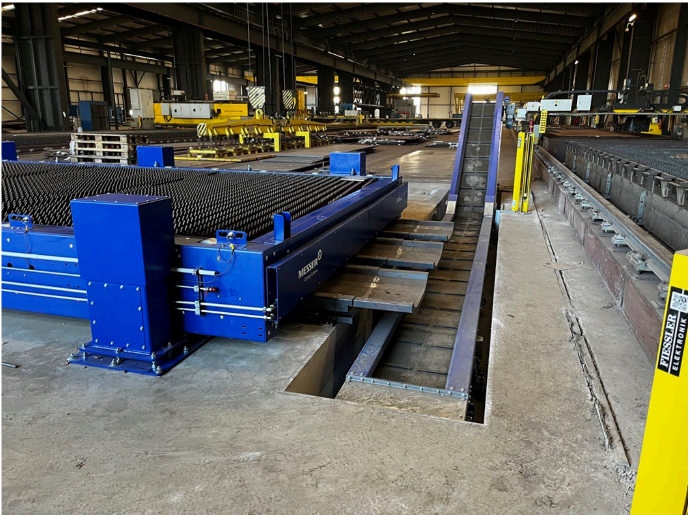
Image 4: Small pieces and slag are carried out of the table by vibrating chutes. The material is automatically transported to a central scrap container via the transverse conveying system, fixed beneath the vibration chutes.
